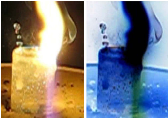
Fig. 7. Rising air bubbles and saltwater drops created at the water–air interface in a test tube of saltwater irradiated by \sim 1 kW of 13.56-MHz RF waves; the rising bubbles are more easily seen in the negative image.
