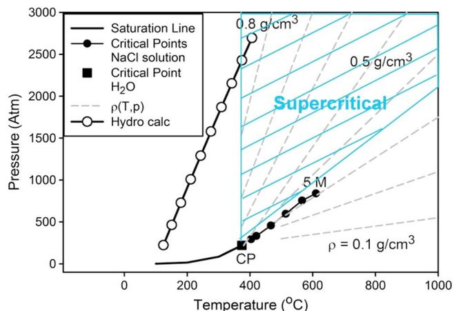
Fig. 2.  $p(T)$  from hydrodynamic surface discharge calculation, with no dissipative losses, along with the water saturation line, critical points for 0.5–5-M saltwater solutions, and fluid density  $\rho(T, p)$  contours.
