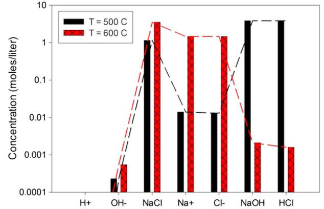
Fig. 5. Equilibrium product concentrations and the amount of water ionized for an initially 5-M NaCl solution comprising only  $\text{H}_2\text{O}$ ,  $\text{Na}^+$ , and  $\text{Cl}^-$ .
