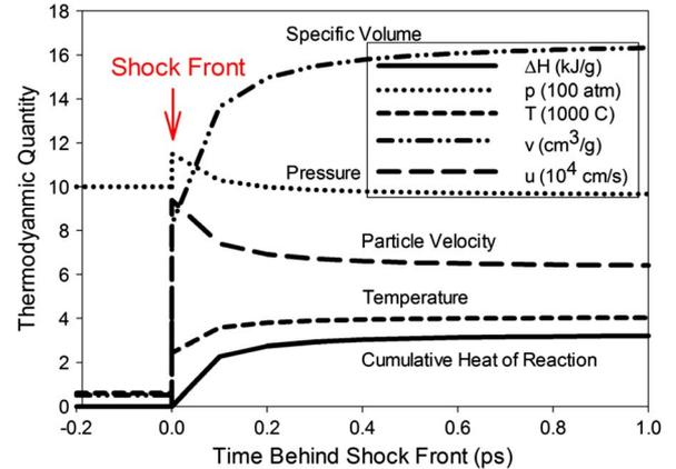
Fig. 8. Time evolution of various thermodynamic properties behind the shock discontinuity in the ZND model. The ambient conditions ahead of the shock front are  $T = 600^\circ\text{C}$ ,  $p = 1000$  atm, and  $u = 0$ .
