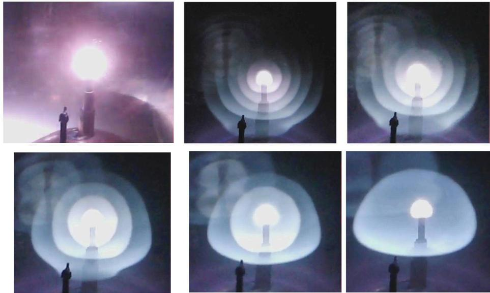
**Figure 10** Sequence of frames from a video of striation formation in a hydrogen. The lighter shifted images are reflections from the wall of the bell jar vacuum chamber.
