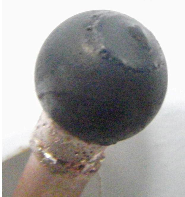
**Figure 9** ¼” (~0.6 cm) diameter iron anode after use in a hydrogen discharge.
