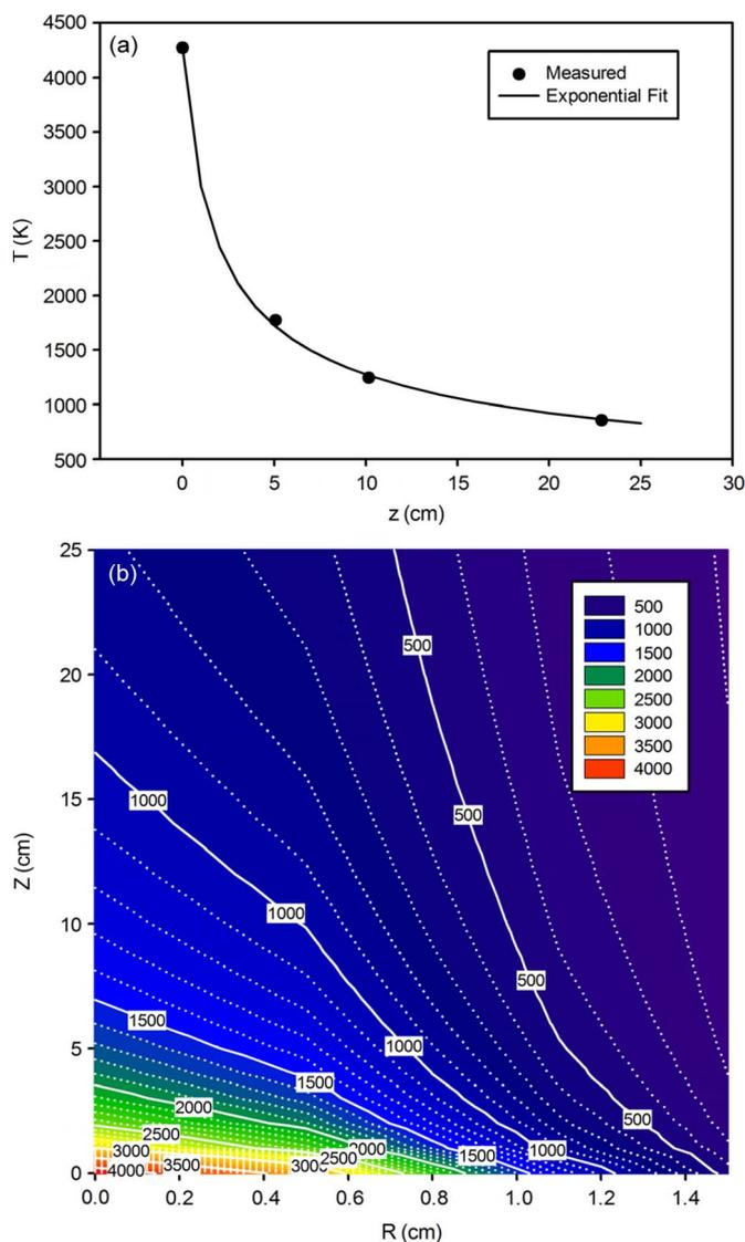
Fig. 3. (a) Vertical temperature profile at the center of a flame produced by a conventional ac arc. (b) Model temperature contours  $T(r, z)$  using the vertical temperature profile of this figure and a Gaussian radial profile.
