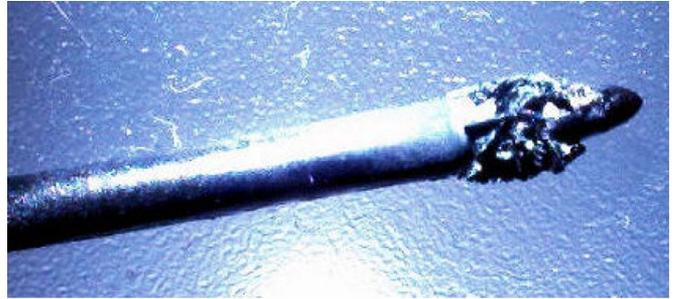
Fig. 2. Ten times microphotograph of  $\text{WCl}_5$  crystals deposited near the tip.
